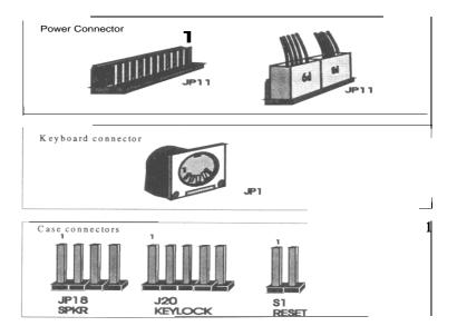
It is imperative that the power connectors be secured in the proper configuration Failure to do so could cause damage to the **board** at power up.
