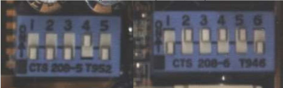
SW2 and SW1 of a K6XV3+/66 with setting 011-110-00010 (66x2.5, 2.8V)
