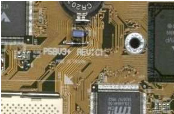
The board revision on the sticker on the outermost ISA plug
