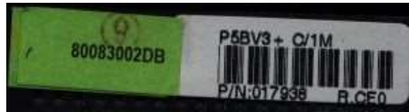
The board revision on the sticker on the outermost ISA plug
