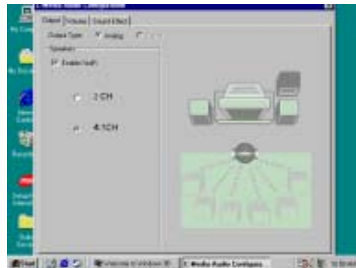
10. When Enabled XearR, you can plug earphone in Speak-Out connector as a Rear speaker, and 2-channel speaker plug in Line-In as Front Speaker to get 4-channel effect
