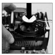
Press the two levers down to fasten the fan. Each lever can be pressed down in only ONE direction.
