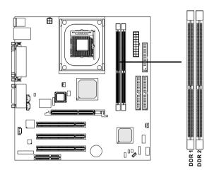
You can install two PC1600/PC2100 DDR SDRAM modules on the DDR DIMM slots (DDR  $1\sim2$ ).
