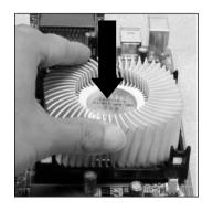
Mount the fan on top of the heatsink. Press down the fan until its four clips get wedged in the holes of the retention mechanism.
