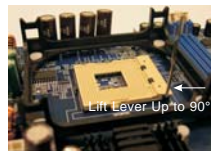
STEP 1: Lift The Socket Lever Up to 90°
