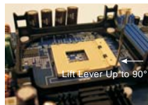
STEP 1: Lift The Socket Lever Up to 90°
