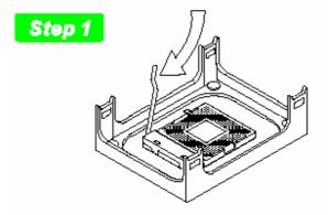
Unlock the socket by pressing the lever sideways, then lift it up to a vertical angle
