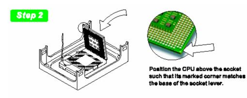
3. Press it firmly on the socket while you push down the socket lever to secure the CPU.
