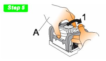
6. Make sure to close the clip levers one at a time. Close the clip lever (1), while holding the top-side of the Fan/Heatsink with your other hand (A). Close the clip lever (2) while holding the top-side of the Fan/ Heatsink with your other hand (B).
