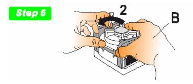
7. Align the Heatsink and clip assembly with the Retention Mechanism and place it on the processor. The Heatsink is symmetrical.
