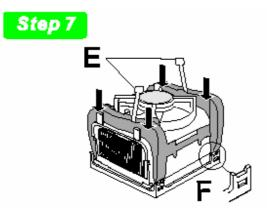
8. With the clip levers in the up position (E), push down on all four clip frame corners to secure to the Retention Mechanism hooks (F). Close the clip levers (G). The levers require force to be completely closed. Connect the processor fan cable connector to the motherboard header.
