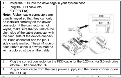
When you first start up your system, go immediately to the Setup Utility to configure the floppy diskette drives that you have installed.
