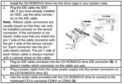
When you first start up your system, the BIOS should automatically detect your CD-ROM/DVD drive. If it doesn't, enter the Setup Utility and configure the CD-ROM/DVD drive that you have installed.
