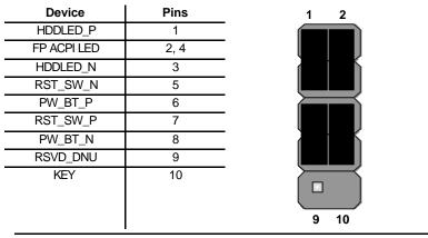
**Note:** The plus sign (+) indicates a pin which must be connected to a positive voltage.
