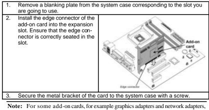
**lote:** For some add-on cards, for example graphics adapters and network adapters, you have to install drivers and software before you can begin using the add-on card.
