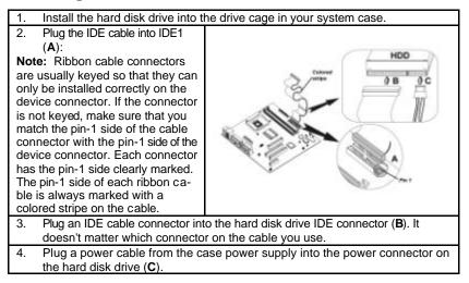
When you first start up your system, the BIOS should automatically detect your hard disk drive. If it doesn't, enter the Setup Utility and use the IDE Hard Disk Auto Detect feature to configure the hard disk drive that you have installed.
