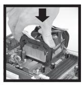
**4.** Press the two levers down to secure the fan. Each lever can be pressed down in only ONE direction.
