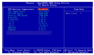
Vcore, vTT 1.25V, 3.3V, Vcc(+5V), +12V, -12V, -5V, 5VSB, Current CPU Temperature, Current CPU Fan Speed, Current System Fan Speed. These items display the current status of all of the monitored hardware devices/components such as CPU voltages, temperatures and all fans' speeds.
