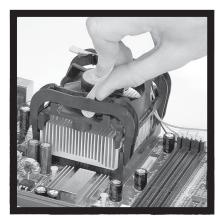
**5.** Connect the fan power cable from the mounted fan to the 3-pin fan power connector on the mainboard.
