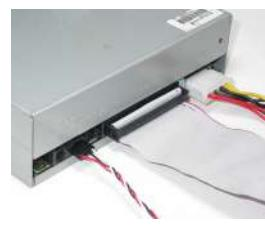
IDE devices enclose jumpers or switches used to set the IDE device as MASTER or SLAVE. Refer to the IDE device user's manual. Installing two IDE devices on one cable, ensure that one device is set to MASTER and the other device is set to SLAVE. The documentation of your IDE device explains how to do this.
