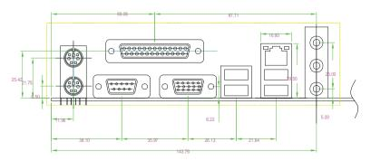
Figure 1: I/O back panel layout
