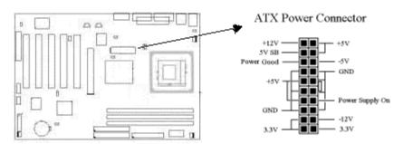
For Pentium 4 Power supply only, you must be insert below power connector in your motherboard.
