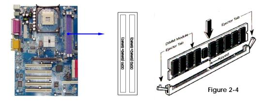
**NOTE!** When you install DIMM module fully into the DIMM socket the eject tab should be locked into the DIMM module very firmly and fit into its indention on both sides.
