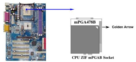
When you put the CPU into the ZIF socket. No force require to insert of the CPU, then press the level to Locate position slightly without any extra force.
