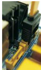
Connect the SATA data cable to one of the orange eSATAII connector (eSATAII_BOTTOM (Port 5))
