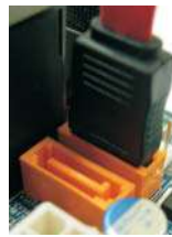
Connect the SATA data cable to one of the orange eSATAII connector (eSATAII_BOTTOM (Port5))
