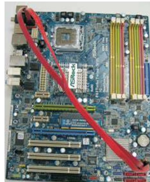
Connect the SATA data cables to both orange eSATAII connectors (eSATAII_BOTTOM (Port5) and eSATAII_TOP (Port4))
