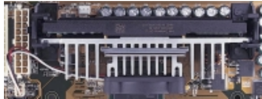
Pentium III (in an SECC2) with heatsink and fan NOTE: The SEPP fan (for Celeron processors) is similar to the SECC2 fan except that the clamping design is different.
