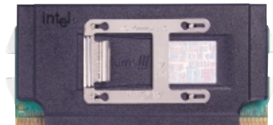
Example of an incorrectly installed retention clip
