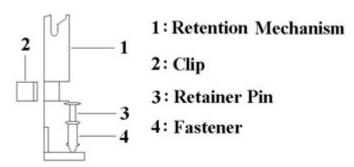
This URM was designed to accommodate 3 types of CPU Form Factor. (SECC, SECCII & SEPP). For Example : Pentium II, Pentium III & Celeron family.
