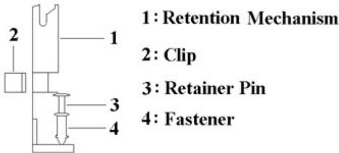
This URM was designed to accommodate 3 types of CPU Form Factor. ( SECC, SECCII & SEPP ). For Example : Pentium II, Pentium III & Celeron family.
