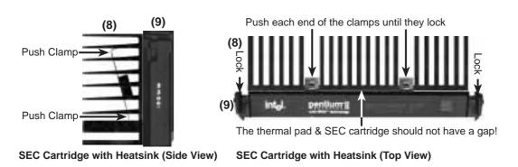
**3. Insert the SEC Cartridge:** Push the SEC cartridge's two locks inward (the preceding picture shows the locks in the outward position and inward in the picture below). With the heatsink facing the motherboard's chipsets, press the cartridge gently but firmly until it is full inserted.
