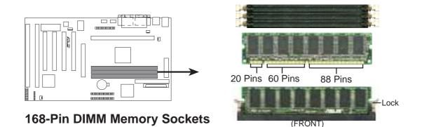
The Dual Inline Memory Module (DIMM) memory modules must be 3.3Volt Unbuffered Synchronous DRAM (SDRAM) or Extended Data Output (EDO). You can identify the type of DIMM module by the illustration below:
