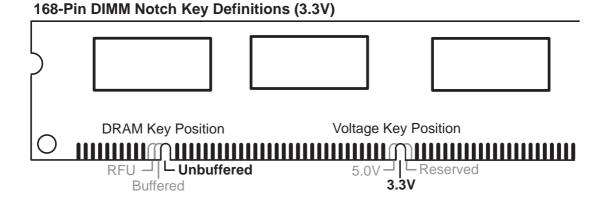
The notch on the DIMM module will shift between left, center, or right to identify the type and also to prevent the wrong type to be inserted into the DIMM slot on the motherboard. You must ask your retailer for the specifications before purchasing. Four clock signals are supported on this motherboard.
