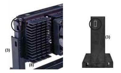
5. Secure the Heatsink: Install the heatsink support base into the motherboard. This is not, however, necessary if you use a heatsink with fan (see next page). The support base is necessary to secure the heatsink (without fan). Secure the heatsink by sliding the heatsink support top bar into the bottom groove of the heatsink until it locks into the heatsink support base posts.
