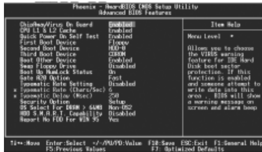
Figure-4 Advanced BIOS Features Menu
