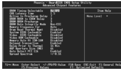
Figure-5 Advanced Chipset Features Menu
