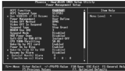
Figure-6 Power Management Setup Menu
