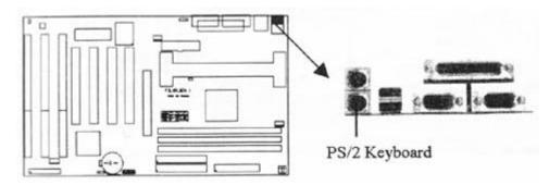
2.4.9 Serial Port (Two 9-pin D-type JCOM)
