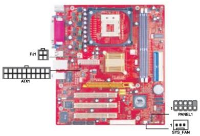
Connect the power connector from the power supply to the **ATX1** connector on the motherboard. The **PJ1** is a +12V connector for CPU Vcore power. If there is a cooling fan installed in the system chassis, connect the cable from the cooling fan to the **SYS\_FAN** fan power connector on the motherboard. Connect the case switches and indicator LEDs to the **PANEL1** header.
