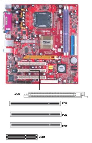
Follow the steps below to install an AGP/CNR/PCI expansion card.
