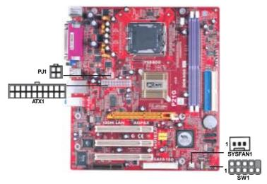
Connect the power connector from the power supply to the **ATX1** connector on the motherboard. The **PJ1** is a +12V connector for CPU Vcore power. If there is a cooling fan installed in the system chassis, connect the cable from the cooling fan to the **SYSFAN1** fan power connector on the motherboard. Connect the case switches and indicator LEDs to the **SW1** header.
