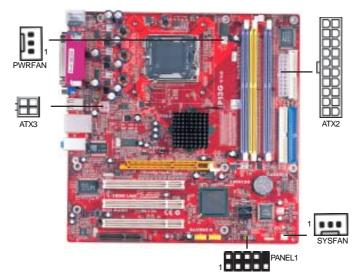
Connect the power connector from the power supply to the **ATX2** connector on the motherboard. The **ATX3** is a +12V connector for CPU Vcore power.
