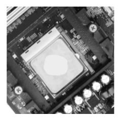
NOTE: The CPU heatsink may have a pre-applied thermal compound. In that case, the silica gel is not required.
