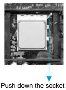
3. When the CPU is in place, press it firmly on the socket while you push down the socket lever to secure the CPU. The lever clicks on the side tab to indicate that it is locked.
