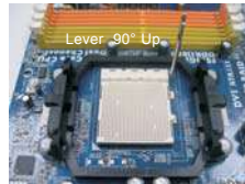
STEP 1: Lift Up The Socket Lever
