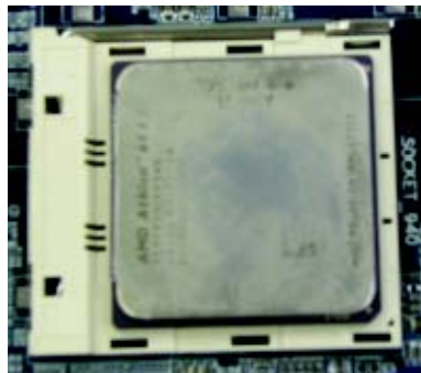
Figure 4. Application of Thermal Grease to the processor.
