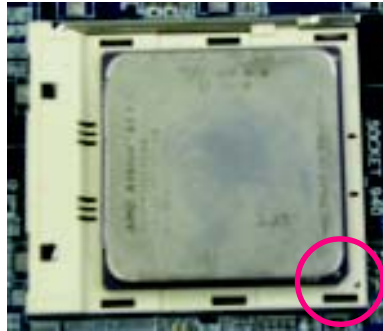
Figure 3. A1 pin location on the Socket and Processor. Move the socket lever to the locked position while holding pressure on the center of the processor.
