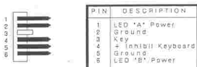
Figure 2-35 Keyboard Lock and Speed Indicator J3
