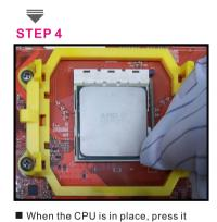
firmly on the socket while you push down the socket lever to secure the CPU. The lever clicks on the side tab to indicate that it is locked.
