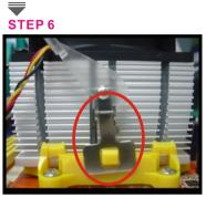
Align the other end of the retention bracket to fasten the cooling set on the top of the retention mechanism
