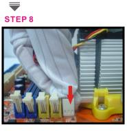
Connect the processor fan cable connector to the CPU\_FAN connector on the motherboard.
