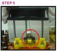
Place the cooling set onto the etention mechanism. Attach one end of the retention bracket to etention mechanism.
