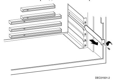
Figure 5-2. Removing a Metal Filler Plate
