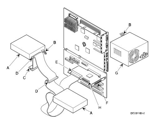
Figure 6-9. SCSI Device Data Cable Connections
