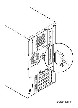
Figure 1-4. Connecting a Local Printer
