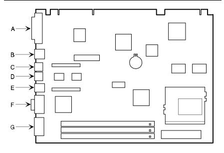
Figure 3-6. Main Logic Board Components (Rear Panel)
