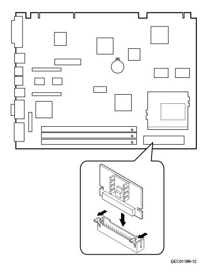
Figure 3-12. Installing a Voltage Regulator
