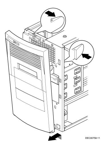
Figure 6-2. Removing the Front Bezel
