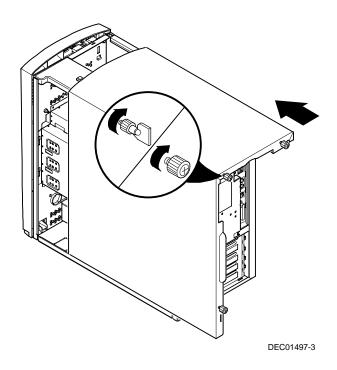
Figure 3-2. Replacing the Outside Cover
