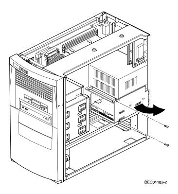
Figure 6-5. Accessing the Internal  $3\frac{1}{2}$ -Inch Device Bay
