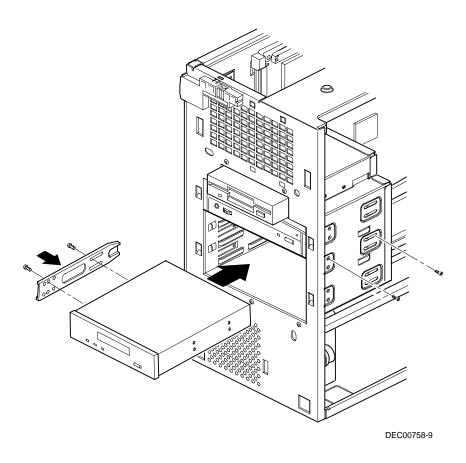
Figure 6-4. Installing 51/4-Inch Device
