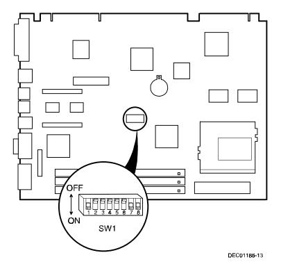
Figure A-1. Main Logic Board Switch Locations
