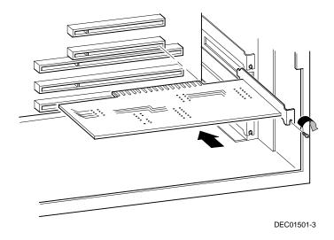
Figure 5-3. Installing an Expansion Board
