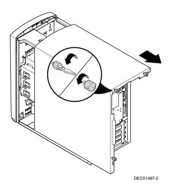
Figure 3-1. Removing the Outside Cover
