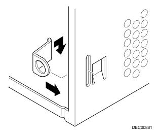
Figure 3-3. Attaching the Hasp
