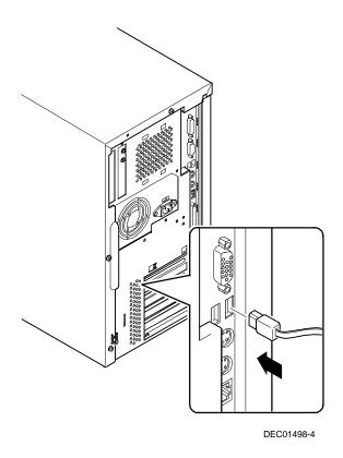
Figure 1-5. Connecting a USB Device
