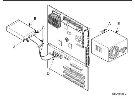
Figure 6-7. Diskette Device Data Cable Connections
