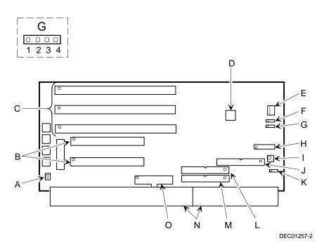
Figure 3-8. System I/O Expansion Card Components and Connectors
