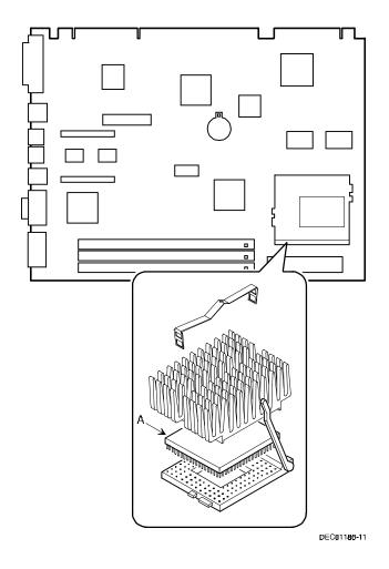
Figure 3-11. Installing a New Processor
