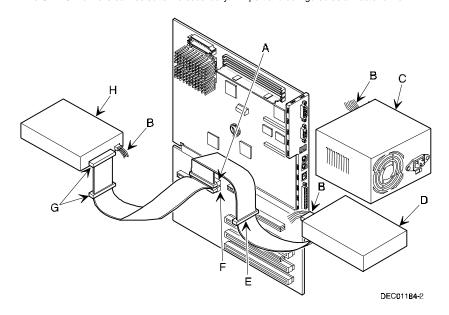
Figure 6-8. IDE Device Data Cable Connections
