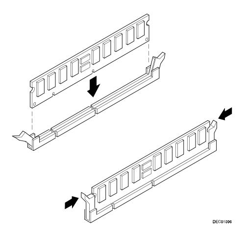
Figure 4-2. Installing a DIMM
