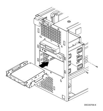
Figure 6-3. Installing a 3½-Inch Device
