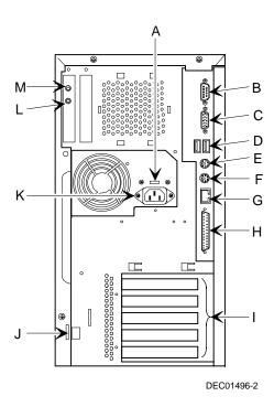
Figure 1-2. Rear Panel Connectors and Voltage Select Switch
