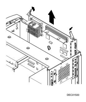
Figure 3-9. Removing the Main Logic Board
