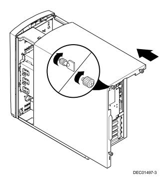
Figure 5-3. Replacing the Outside Cover
