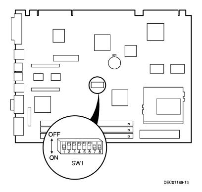
Figure 5-10. Main Logic Board Switch Locations
