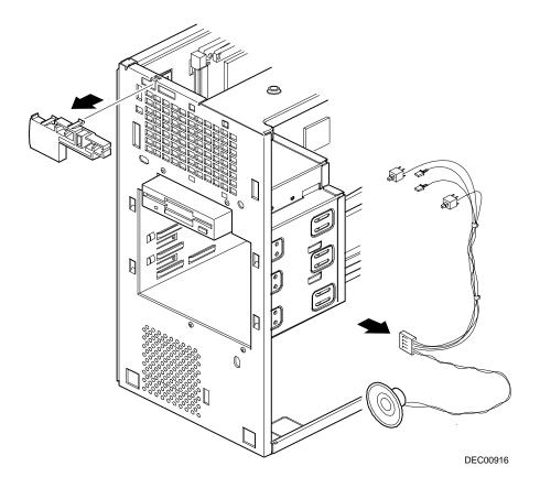
Figure 5-15. Removing the Control Panel Assembly and Cable
