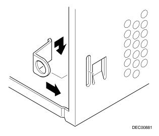
Figure 5-4. Attaching the Hasp
