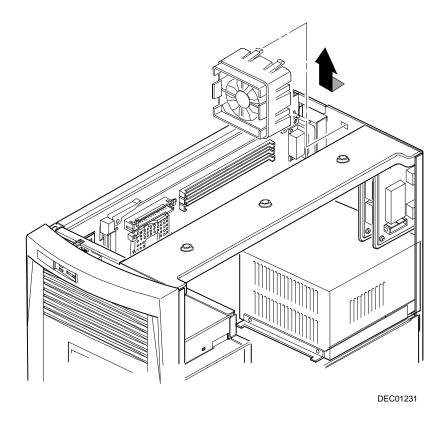
Figure 5-17. Removing the Top-Rear Fan Assembly
