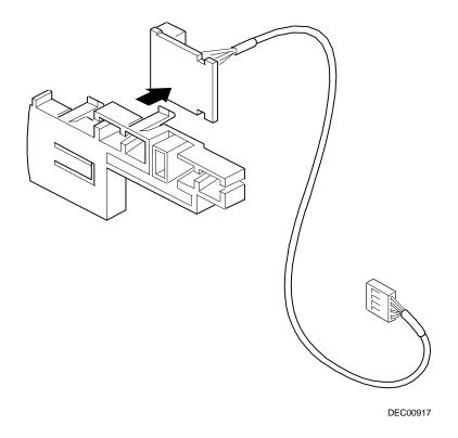
Figure 5-18. Removing the Wire Assembly, Headphone/Microphone
