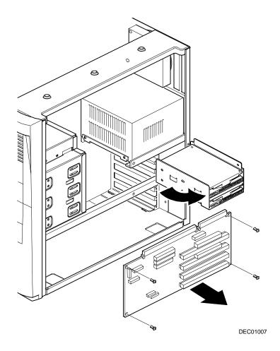
Figure 5-12. Removing the Backplane
