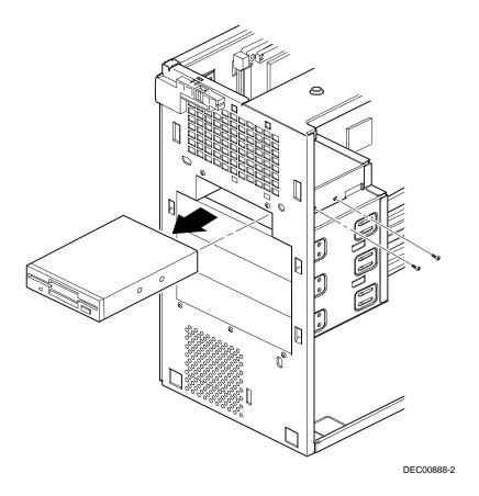
Figure 5-19. Removing the Diskette Drive
