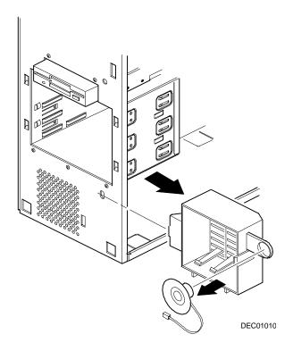
Figure 5-16. Removing the Option Card Guide and Speaker Assembly
