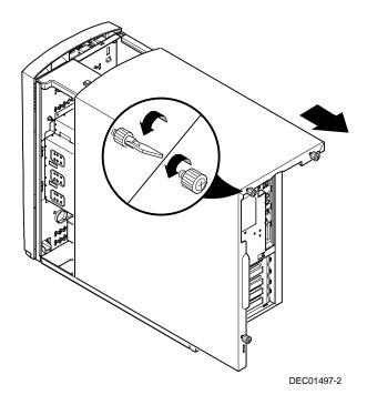
Figure 5-2. Removing the Outside Cover
