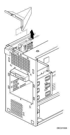
Figure 5-14. Removing the Front Air Duct
