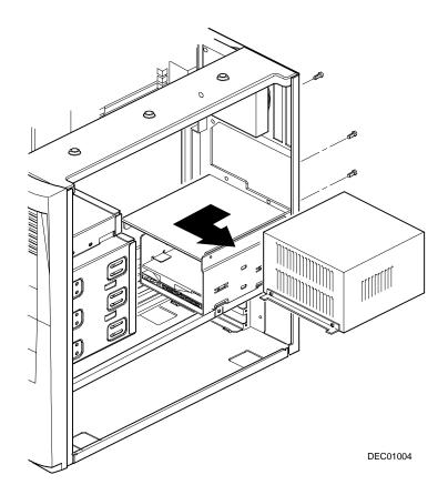
Figure 5-13. Removing the Power Supply
