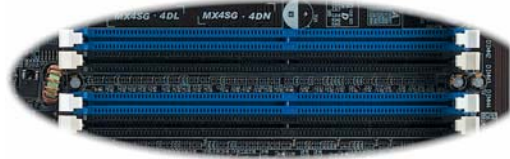
128-bit DDR Dual Channel Memory module (For MX4SG-4DL and MX4SG-4DN only)
