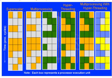
The figure below represents how Hyper-Threading saves time when it
