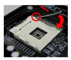
2. Locate Pin 1 in the socket and look for mark on the CPU upper interface. Match Pin 1 and cut edge, then insert the CPU into the socket.
