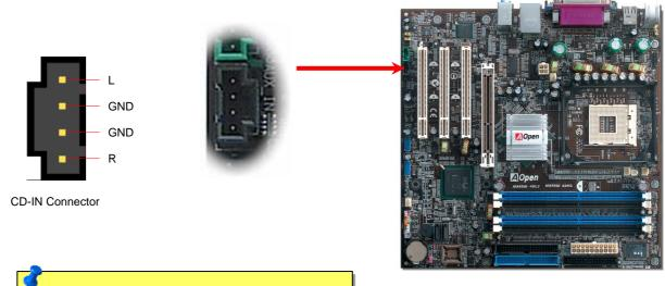
**Note:** Though some of the latest versions of Windows support "Digital Audio" through IDE bus. However, in order to use Open Jukebox player, which is driven under BIOS, it is a **MUST** to connect audio cable to CD-IN connector on the motherboard.
