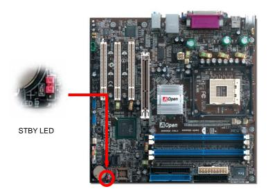
**Warning:** Do not install or remove the DIMM module or others devices when the STBY LED lights on.
