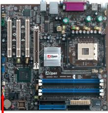
Attach the power LED, Keylock, speaker, power and reset switch connectors to the corresponding pins. If you enable "Suspend Mode" item in BIOS Setup, the ACPI & Power LED will keep flashing while the system is in suspend mode.
