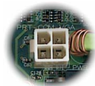
4-Pin 12V ATX 电源接头
