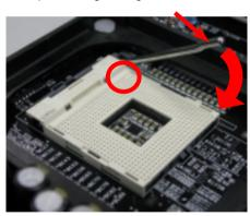
2. Locate Pin 1 in the socket and look for a cut edge on the CPU upper interface. Match Pin 1 and cut edge, then insert the CPU into the socket.
