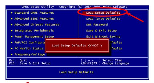
Warning: Please avoid of using "Load Turbo Defaults", unless you are sure your system components (CPU, DRAM, HDD, etc.) are good enough for turbo setting.
