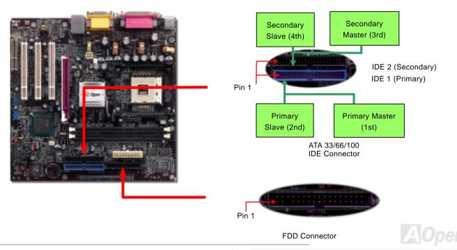
IDE1 is also known as the primary channel and IDE2 as the secondary channel. Each channel supports two IDE devices that make a total of four devices. In order to work together, the two devices on each channel must be set differently to **Master** and **Slave** mode. Either one can be the hard disk or the CDROM. The setting as master or slave mode depends on the jumper on your IDE device, so please refer to your hard disk and CDROM manual accordingly.
