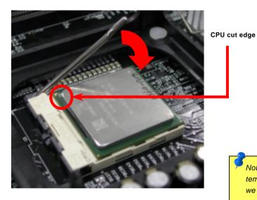
**Note:** If you do not match the CPU socket Pin 1 and CPU cut edge well, it may damage the CPU.
