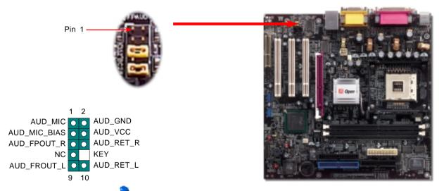
**Note:** Please remove the jumper cap from the Front Panel Audio Connector before you connect the cable. Do not remove this yellow jumper cap if housing without an audio port on the front panel.
