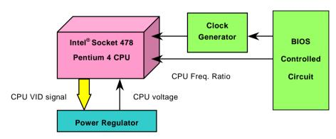
(Automatically generates CPU voltage)
