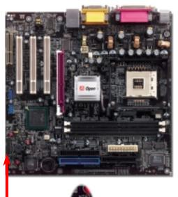
Attach the power LED, Keylock, speaker, power and reset switch connectors to the corresponding pins. If you enable "Suspend Mode" item in BIOS Setup, the ACPI & Power LED will keep flashing while the system is in suspend mode.
