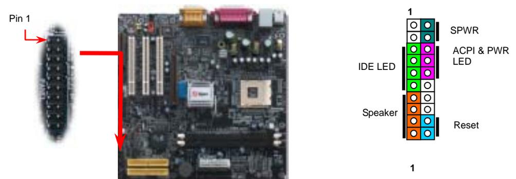
Attach the power LED, speaker, and reset switch connectors to the corresponding pins. If you enable "Suspend Mode" item in BIOS Setup, the ACPI & Power LED will keep flashing while the system is in suspend mode.
