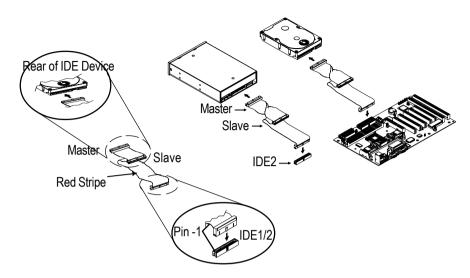
The primary channel has priority to the secondary channel. Within each channel, the two different devices are distinguished by master and slave relationship. The master device has priority over the slave device. (Refer to illustration on the below)
