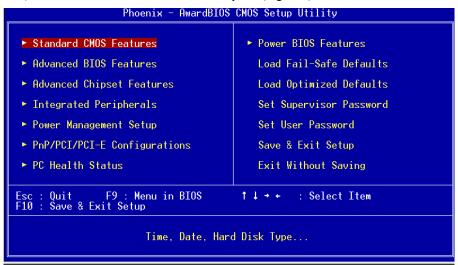
Figure 1: CMOS Setup Utility
