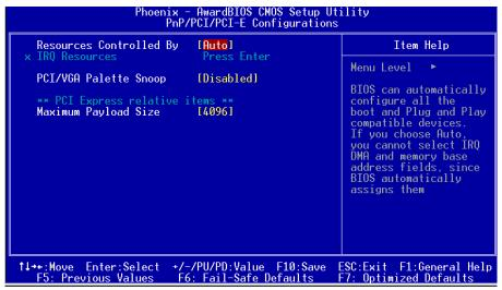
Figure 7: PNP/PCI/PCI-E Configuration Setup
