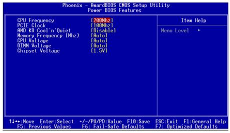
Figure 9: Frequency/Voltage Control
