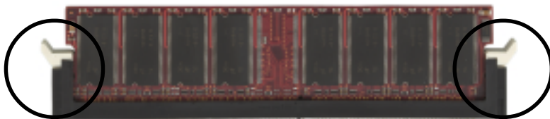
Figure 8 - DIMM module clip after installation
