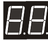
80 Port Debug 7-segment LED display (Refer to Appendix D for POST codes)
