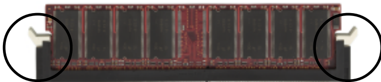
Figure 10 - DIMM module clip after installation
