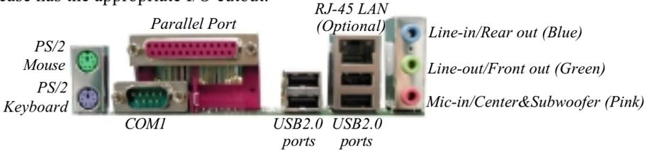
Figure 3: I/O ports
