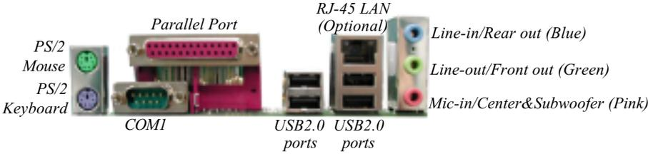
Figure 12 - I/O Ports
