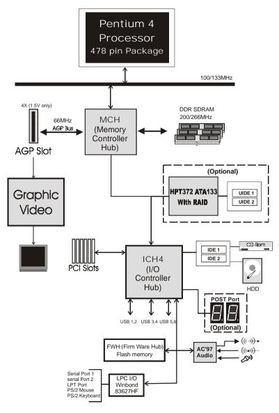
Figure 5: System Block Diagram
