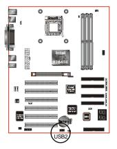
**USB2:** USB port header pins for share with four USB ports.
