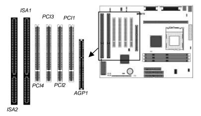
Use the AGP1 slot to install an AGP graphics adapter. Use the PCI slots to install 32-bit PCI expansion cards. Use the ISA slots to install legacy 8/16-bit expansion cards.
