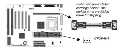
2. The Slot-1 is installed with a cartridge holder. The upright struts of the cartridge holder are folded down for shipping. Pull the struts upwards so that they are in the upright position.
