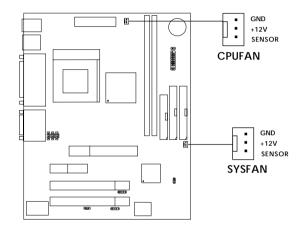
**CPUFAN**: Processor Fan **SYSFAN**: System Fan
