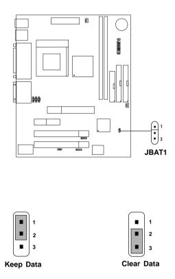
**Note:** You can clear CMOS by shorting 2-3 pin, while the system is off. Then, return to 1-2 pin position. Avoid clearing the CMOS while the system is on, it will damage the mainboard. Always unplug the power cord from the wall socket.
