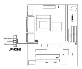
Mono\_Out is connected to the Modem Speaker Out connector. Phone\_In is connected to the Modem Microphone In connector.
