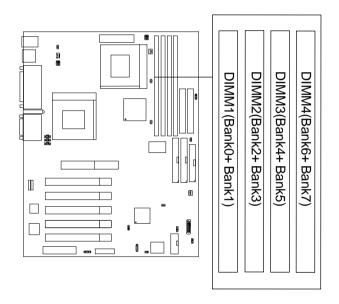
There are three kinds of DIMM specification supported by this mainboard: PC133, PC100 and PC66. If you use 66MHz CPU Bus Frequency, these four DIMM Specs. is supported. If you use 100 MHz CPU Bus Frequency, only PC100 DIMM Specs. is supported.If you use 133 MHz CPU Bus Frequency, only PC133 DIMM Specs. is supported.
