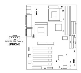
Mono\_Out is connected to the Modem Speaker Out connector. Phone\_In is connected to the Modem Microphone In connector.
