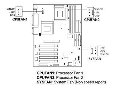
For fans with fan speed sensor, every rotation of the fan will send out 2 pulses. System Hardware Monitor will count and report the fan rotation speed.
