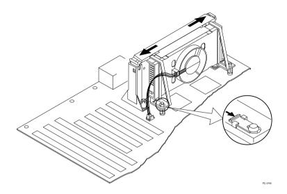
Step 7: Lock the Processor Locks and Heat Sink Support Locks
