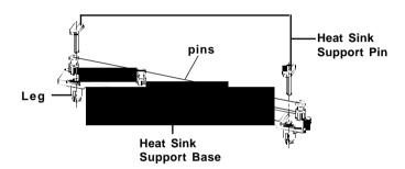
Push the Heat Sink Support Base onto the mainboard, until you hear a click sound. Check for a perfect fit.
