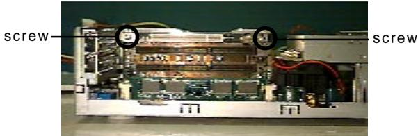
Secure the MS-5296 riser card into the Chassis with screws.
