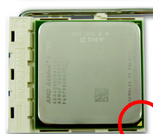
Fig.2 Pin 1 location on the socket and processor. Gently place the CPU into position making sure that the CPU pins fit perfectly into their holes. Once the CPU is positioned into its socket, place one finger down on the middle of the CPU and gently press the metal lever back into its original position.
